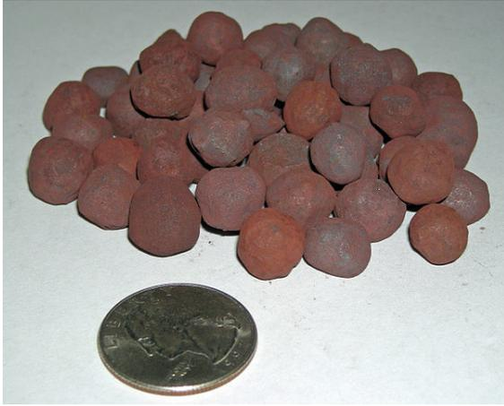
*Processed taconite pellets with reddish surface oxidation as used in the steelmaking industry, with a US Quarter (diameter: 24 mm (0.96 in)) shown for scale*
