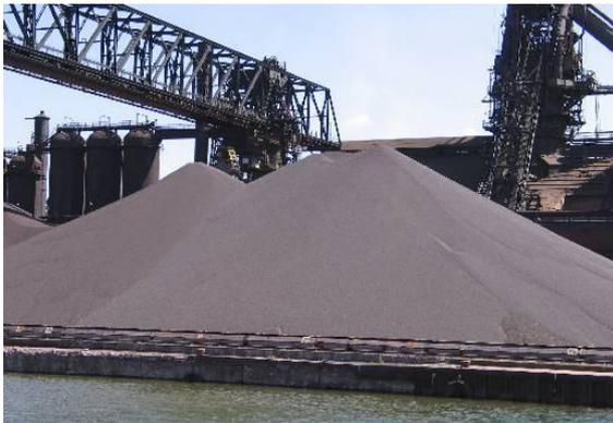
*This stockpile of iron ore pellets will be used in steel production.*
