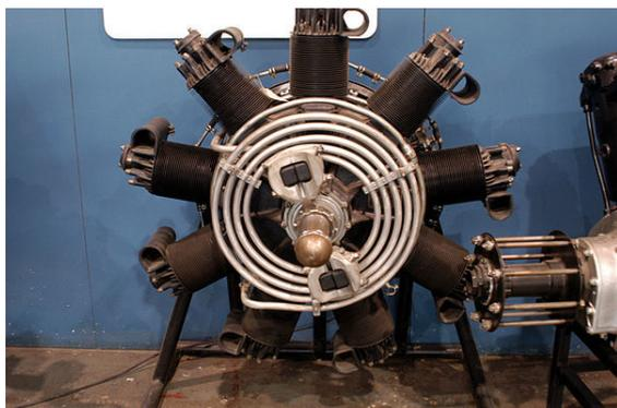
*Packard DR-980 9-cylinder diesel aircraft engine*
