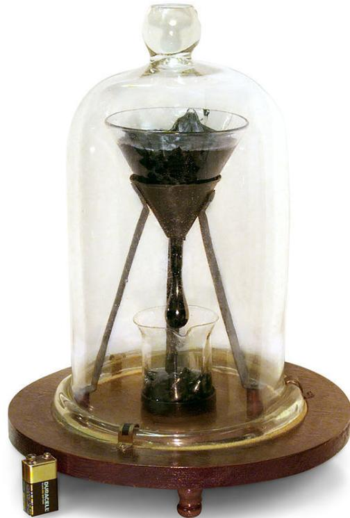
*The University of Queensland pitch drop experiment, demonstrating the viscosity of asphalt/bitumen*
